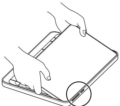
Align the power button and volume buttons with the holes.
